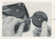
7 Thread the end of the film into the slot in the take-up spool core; then wind the slack film, black side out, onto the take-up spool by turning the spool in the direction of the arrow. If the film binds between the spool flanges, the flanges are bent; straighten them with your fingers.
