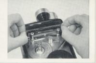
5 Let the film follow the line with the arrow from the bottom of the film spool to the gate. Slide the film down into the gate; that is, between the pressure pad and aperture plate (pointed out in 3 at left).
