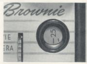
12 After the cover is on and locked, hold the exposure lever down until 25 on the dial of the footage indicator is at the index. Now you can take pictures.
