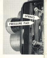
Carefully clean the polished surfaces of the gate and pressure pad with a slightly moist cloth; do not scrape the track with any metallic object. Then polish the parts with a clean, soft, lintless cloth. Make sure the parts are dry.
