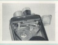
6 Push the film all the way down, at the top of the camera first; then at the bottom. Pull the film through the gate until there are approximately 9 inches below the gate.
