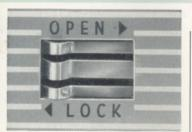
11 Replace the cover and lock it by pushing the latch to the LOCK end of its slot. If the cover does not go on, check to see that both spools are seated properly on the spindles.
