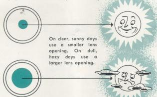
The lens opening marked 1.9 is the largest and admits the most light. Each succeeding marked opening from 1.9 to 16 lets through only one half as much light. Each marked lens opening is called a "stop"; the white dot between marked openings indicates a half stop.
