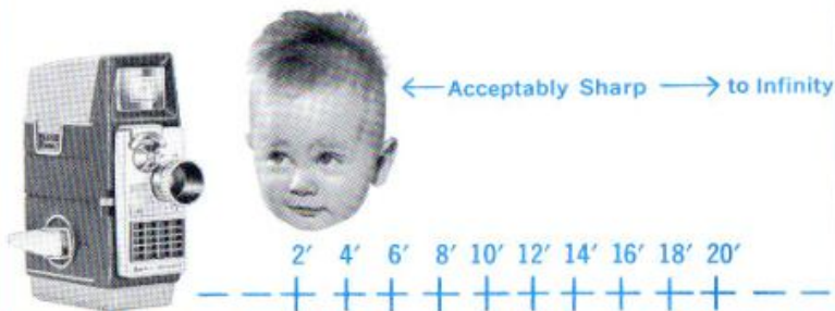
Example: 10mm lens reading f/8 subject in focus from 2 FEET TO INFINITY
