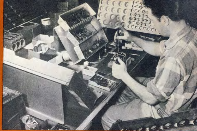
Sub-assemblies are brought together in camera case in one of the first production steps. Tiny screw being driven was produced by Keystone's own screw machines.
