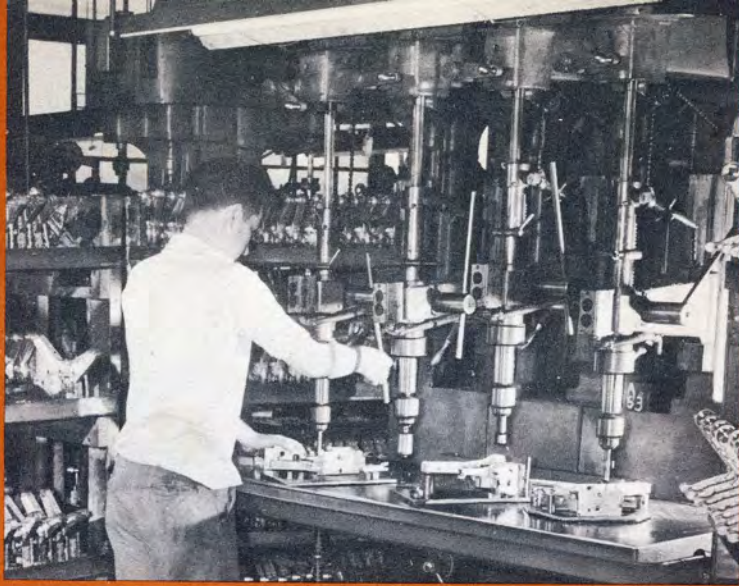
This automatic drilling machine that performs several successive operations is one of the largest of its kind.
