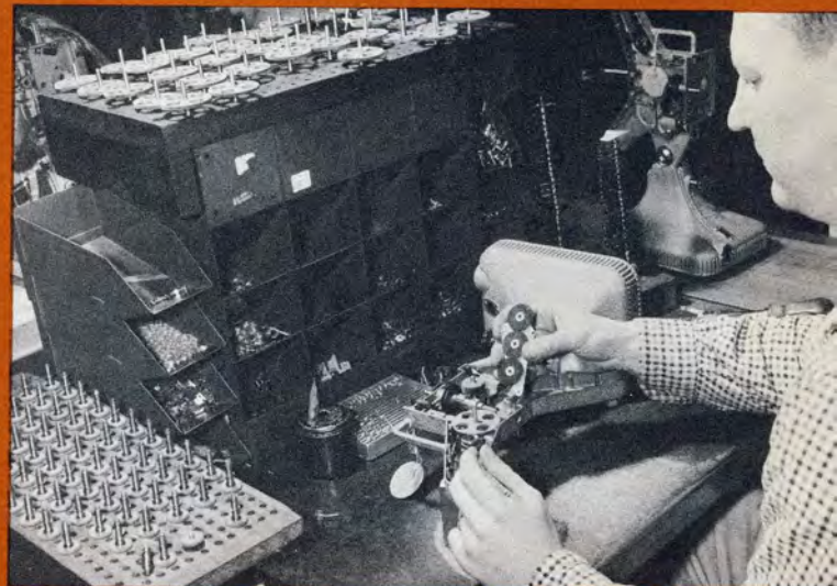
Fitting gears in the projector arm. Precision-gear film wind is an exclusive feature in many Keystone models.
