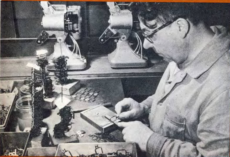
Projection "finger" honed by unhurried hand process gives a fit even finer than obtainable from the most precise machine.
