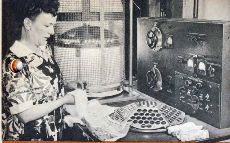
All projector-condenser lenses are coated, and polished by hand in Keystone's own coating dept.
