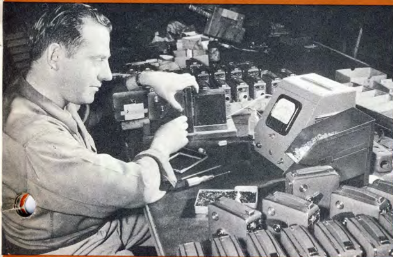
Setting governor speed of camera with electronic meter. Every latest device is used to control the quality of Keystone products from small electrical machines like this to huge automatic multiple-operation machines.
